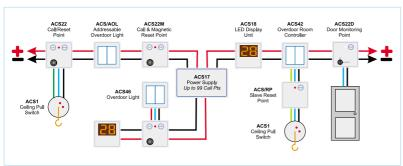
up to 32 call points – there are countless applications where a small or medium sized call system is required. The ACS27 offers a perfect solution. This cost effective panel is a combined PSU and display in one unit, allowing up to 32 call points to be powered from the central panel. The ACS27 has the additional benefit of Mute and Reset buttons which can be disabled if not required.
